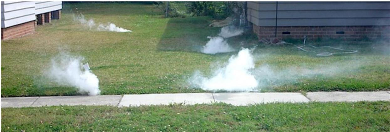
*In this photo, a defect in an underground sewer pipe is allowing smoke to escape up through the ground.*
