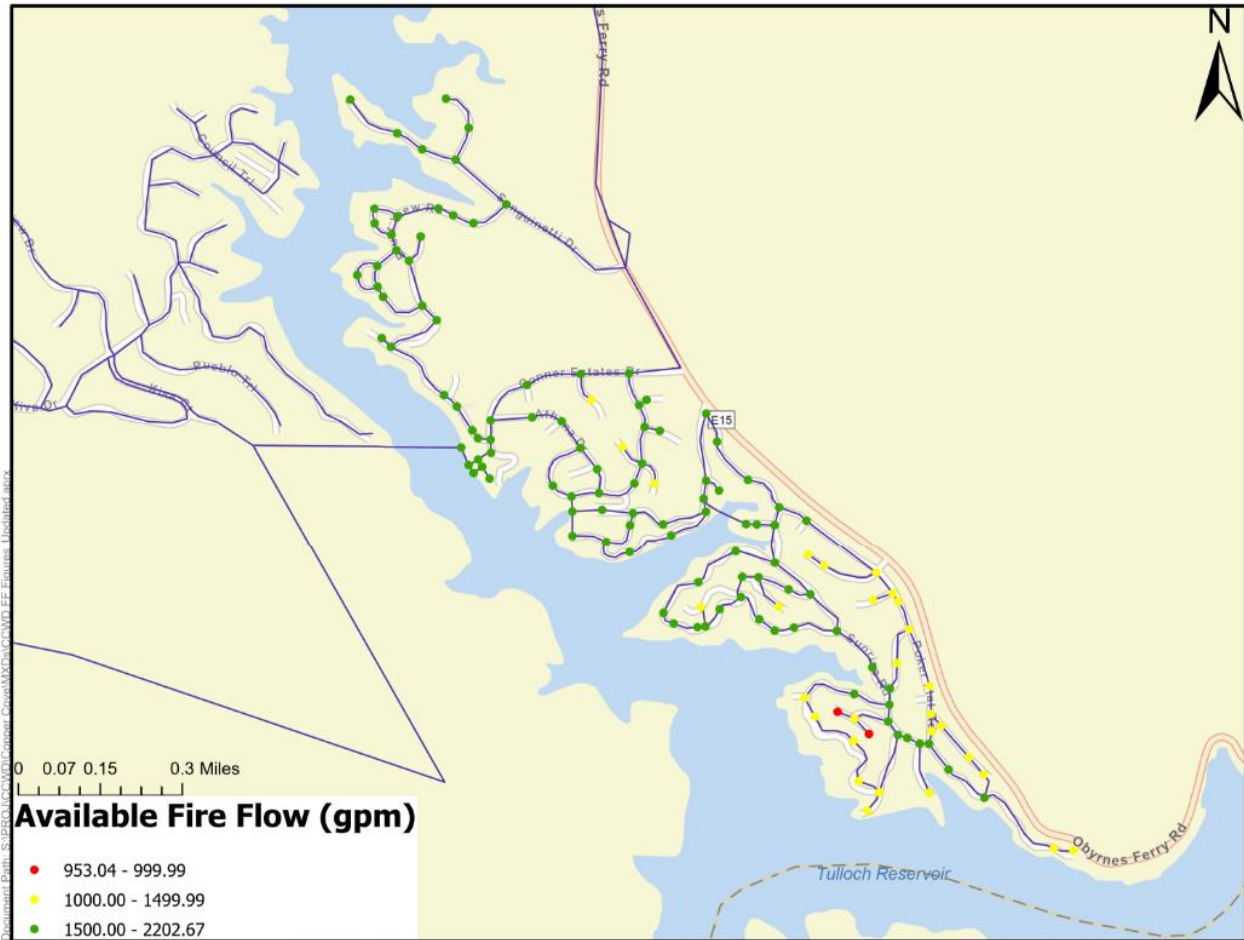
Figure 8. Alternative 2A - 12" Transmission Main
