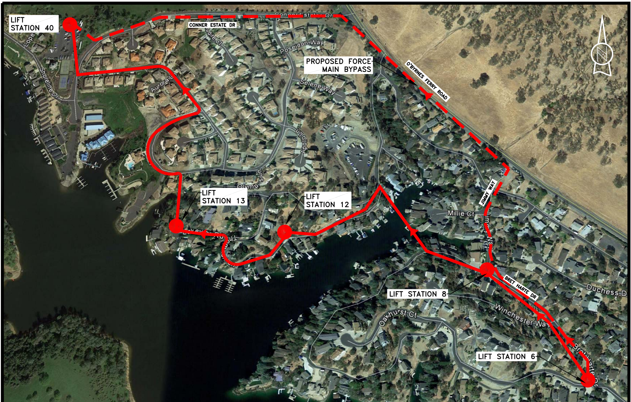
LIFT STATION 6, 8, 12 & 13 FORCE MAIN PROPOSED ALIGNMENT (FIGURE-1)
