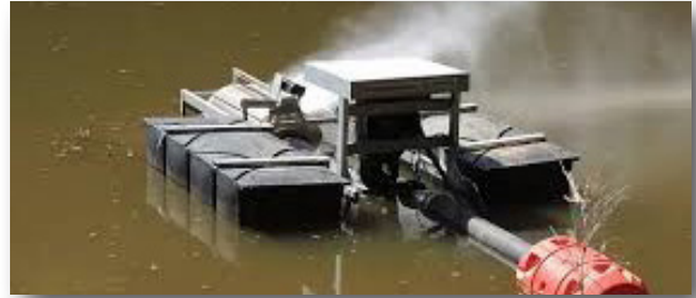
↑ FIGURE 1 - FLOATING INTAKE
